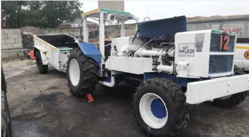
Tractor-trailer for transporting building material underground
