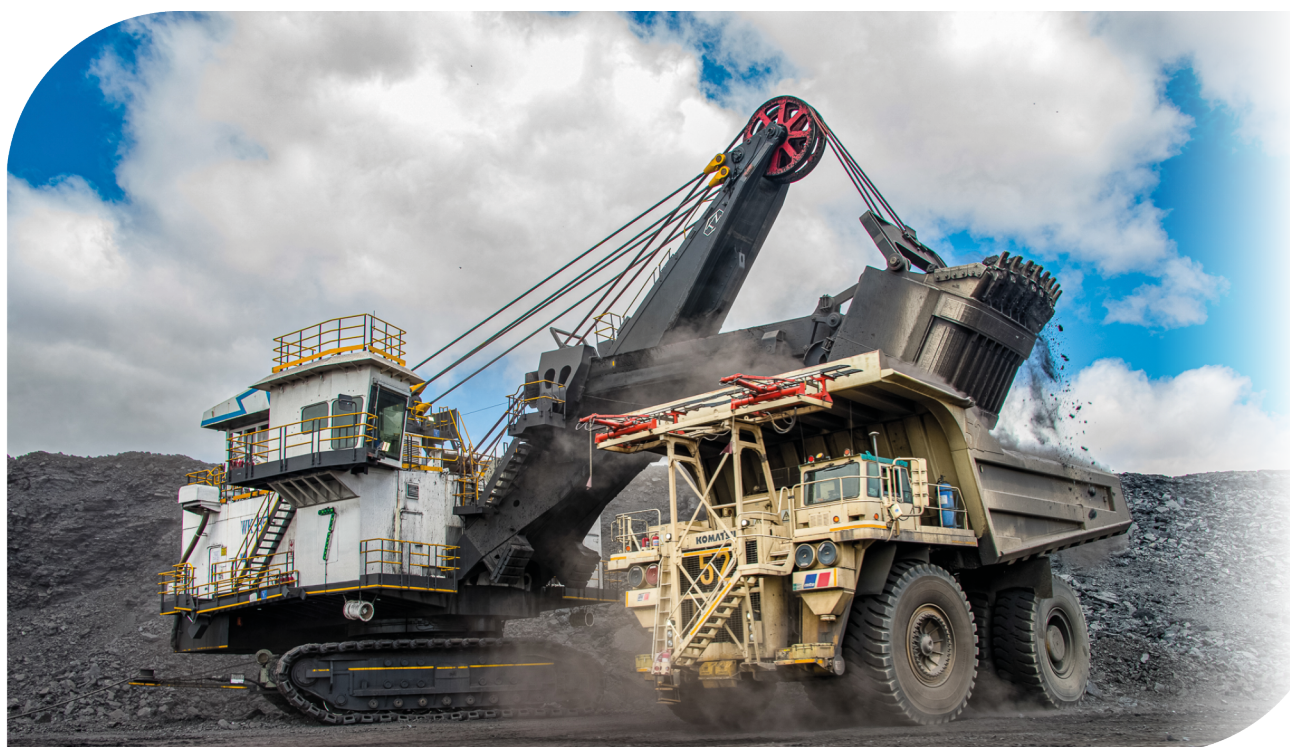
Rope shovel loading coal at Grootegeluk
